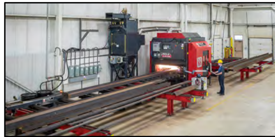
Fully automated 6 axis structural processor
