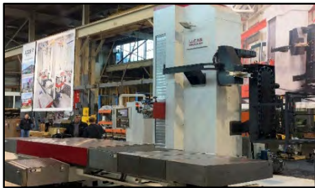
Boring up to 120" x 98" x 29" with Cat50 Spindle
