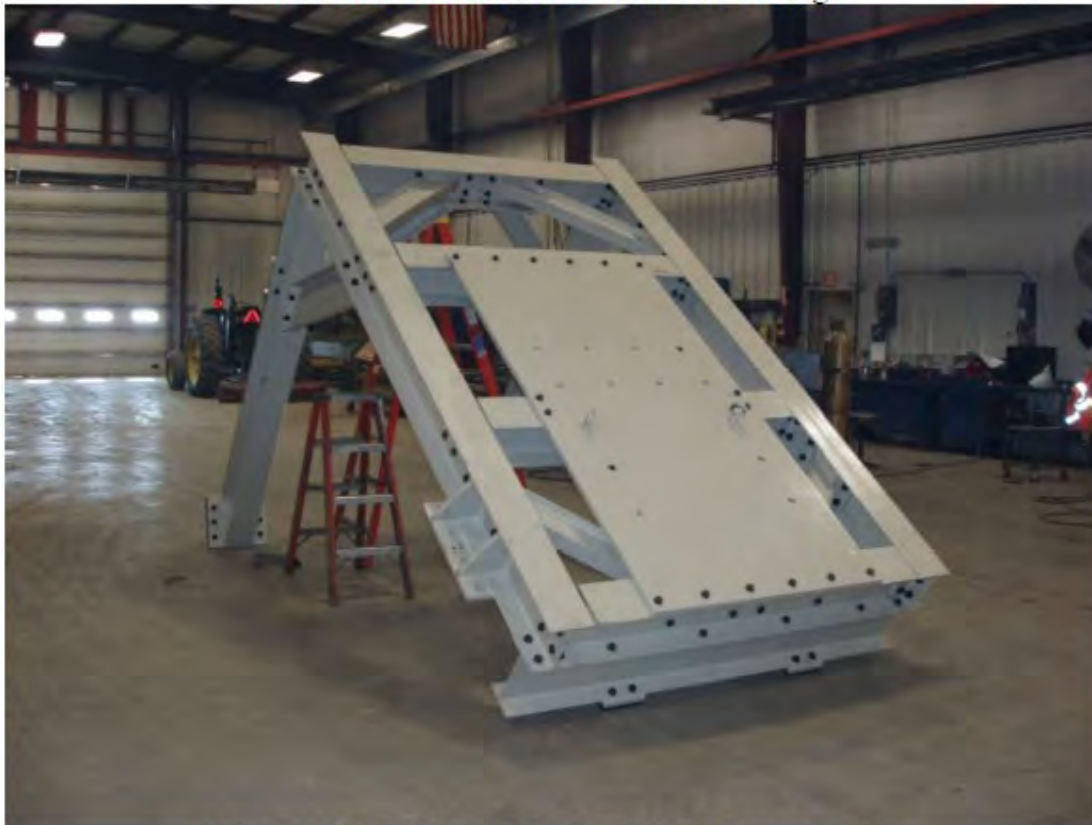
Fabricated Steel Frame for Boulder Breaker Project
