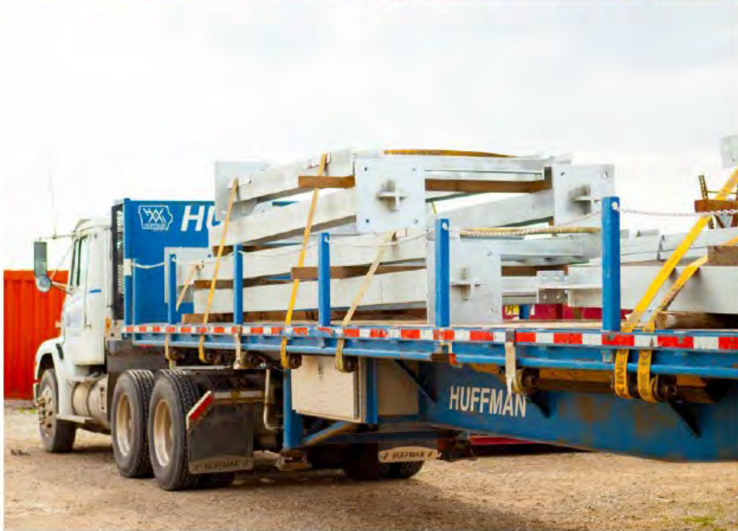
Heavy structural steel --- Shown is large industrial pipe rack steel hot dipped galvanized
