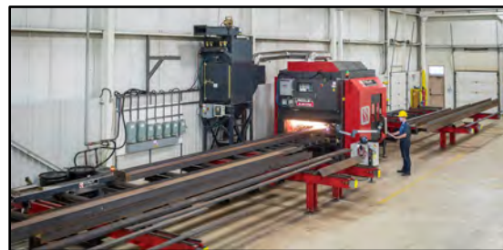
Fully automated 6 axis structural processor
